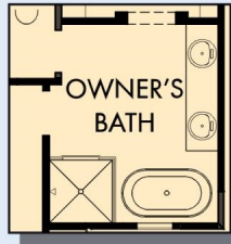
OWNER'S BATH OPTIONAL FREE STANDING TUB WITH SEPARATE SHOWER AT OWNER'S BATH
